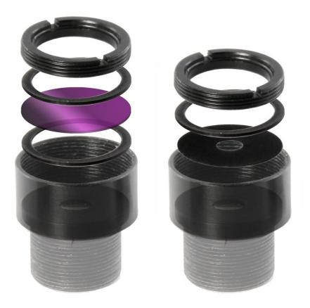
The filter holder FAM12D14H08 allows add Filters\* to standard S-Mount (M12x0.5) Lenses and to modify the F# of Front Iris lenses. This set consists of one holder, two nylon rings and one lock ring.
