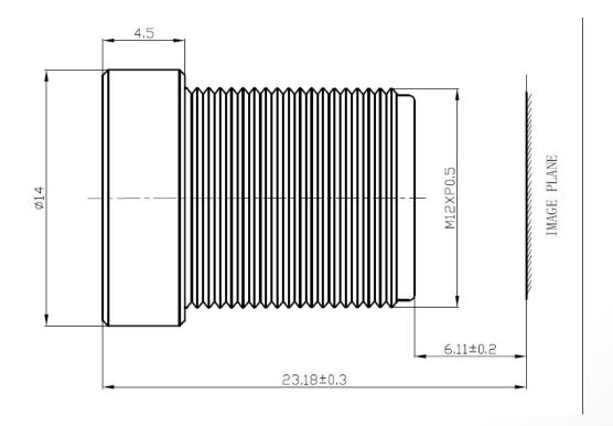
The S-Mount lens Lensagon BT6020DNC is suitable for common sensors up to 1 megapixel with an image format of 1/3 inch. It is characterized by a particularly high light intensity.
