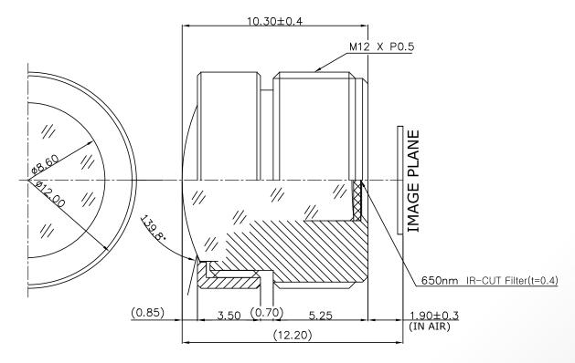
The S-Mount lens Lensagon BMK2320C is suitable for common sensors up to 1.3 megapixel with an image format of 1/3 inch. It is characterized by a particularly high light intensity. Construction: 6 elements (1ASP glass / 5G)
