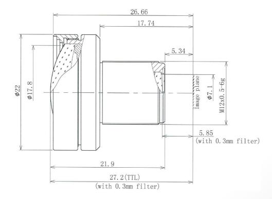
The S-Mount lens Lensagon BM3516NDC is suitable for common sensors up to 1.3 megapixel with an image format of 1/3 inch. It is characterized by a particularly high light intensity. CRA @R=3mm: 9,8° EP Position ab 1 Linse: 8,99.
