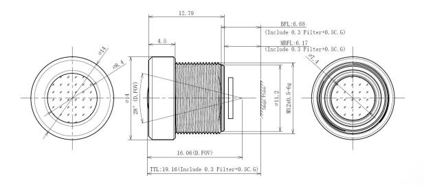
The S-Mount lens Lensagon BM12018V2C is suitable for sensors below 1 megapixel with an image format of 1/3 inch. It is characterized by a particularly high light intensity.
