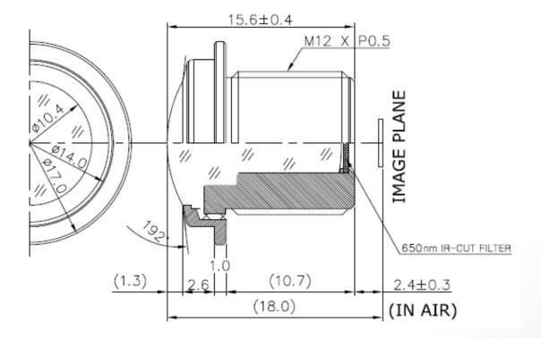
The S-Mount lens Lensagon BK1220C is suitable for sensors below 1 megapixel with an image format of 1/4 inch. It is characterized by a particularly high light intensity.
