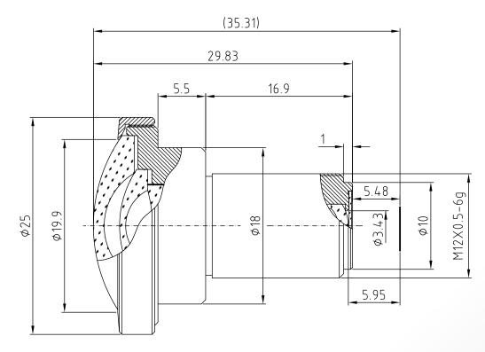
The Fisheye S-Mount lens Lensagon BF5M11920C is suitable for common sensors up to 5.00 megapixel with an image format of 1/3.2 inch. It is characterized by a particularly high light intensity. Effective Aperture: 19.9mm (Front)
