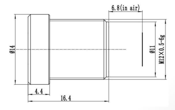
The S-Mount lens Lensagon BE5M8020S125 is suitable for common sensors up to 5 megapixel with an image format of 1/2.5 inch. It is characterized by a particularly high light intensity.
