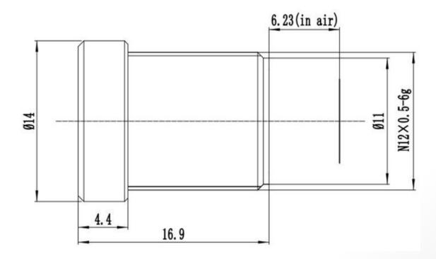
The S-Mount lens Lensagon BE5M12020S125 is suitable for common sensors up to 5 megapixel with an image format of 1/2.5 inch. It is characterized by a particularly high light intensity.
