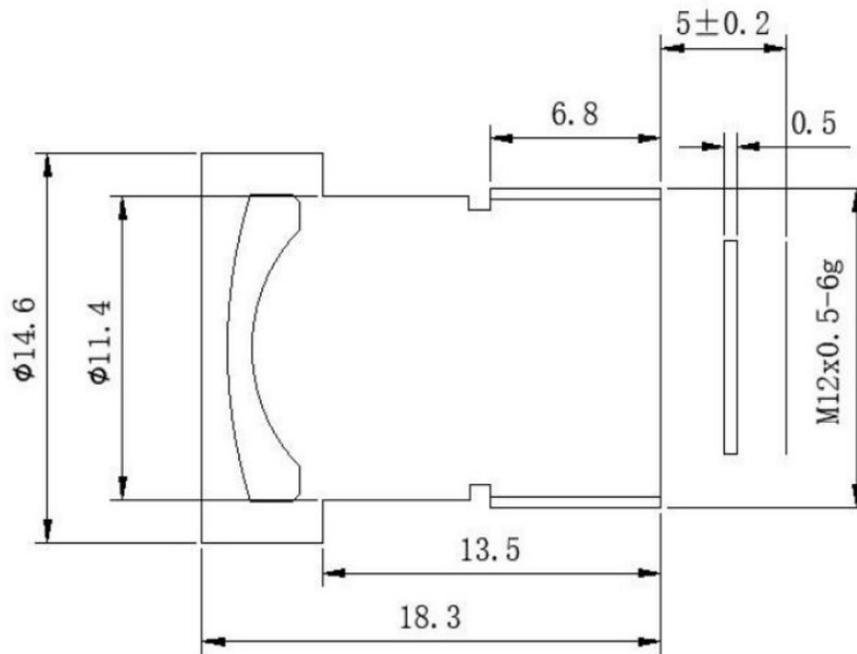
The S-Mount lens Lensagon B6M6156S12 is suitable for current sensors up to 6.00 megapixel with an image format of 1/2 inch.
