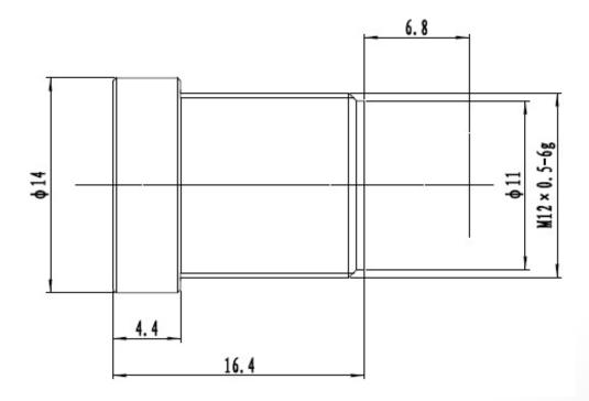
The S-Mount lens Lensagon B5M8020 is suitable for common sensors up to 5.00 megapixel with an image format of 1/2.5 inch. It is characterized by a particularly high light intensity.
