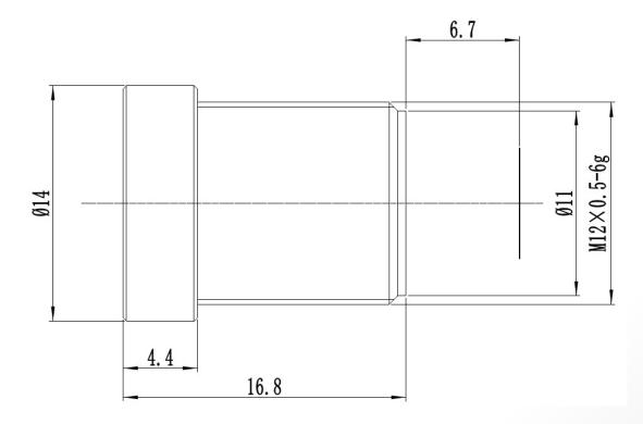
The S-Mount lens Lensagon B5M6020 is suitable for common sensors up to 5 megapixel with an image format of 1/2.5 inch. It is characterized by a particularly high light intensity.
