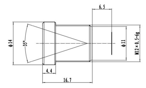
The S-Mount lens Lensagon B5M12020C is suitable for common sensors up to 5 megapixel with an image format of 1/2 inch. It is characterized by a particularly high light intensity.
